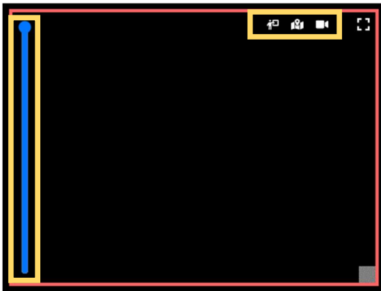
Closeup of a window on the MapBlender workspace. Using the slider on the left controls the translucency, the three buttons in the top-right corner affect the blend mode.
